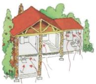
Radon in soil gas is the main source of radon problems. Pathways for radon to enter a building include cracks in the slabs and walls, the expansion joints between floor and walls, porous concrete block walls, open sump pits, crawlspaces and openings around utility penetrations. Some buildings have other pathways for radon to enter a building such as sub-slab utility tunnels and heating, ventilating and air conditioning (HVAC) ducts.
