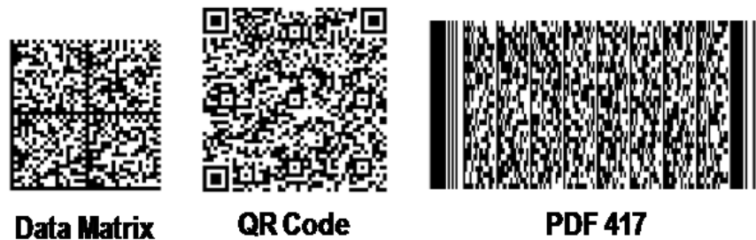
FIGURE 1 - Examples of Data Matrix, QR Code and PDF 417 Two-dimensional (2D) symbologies
