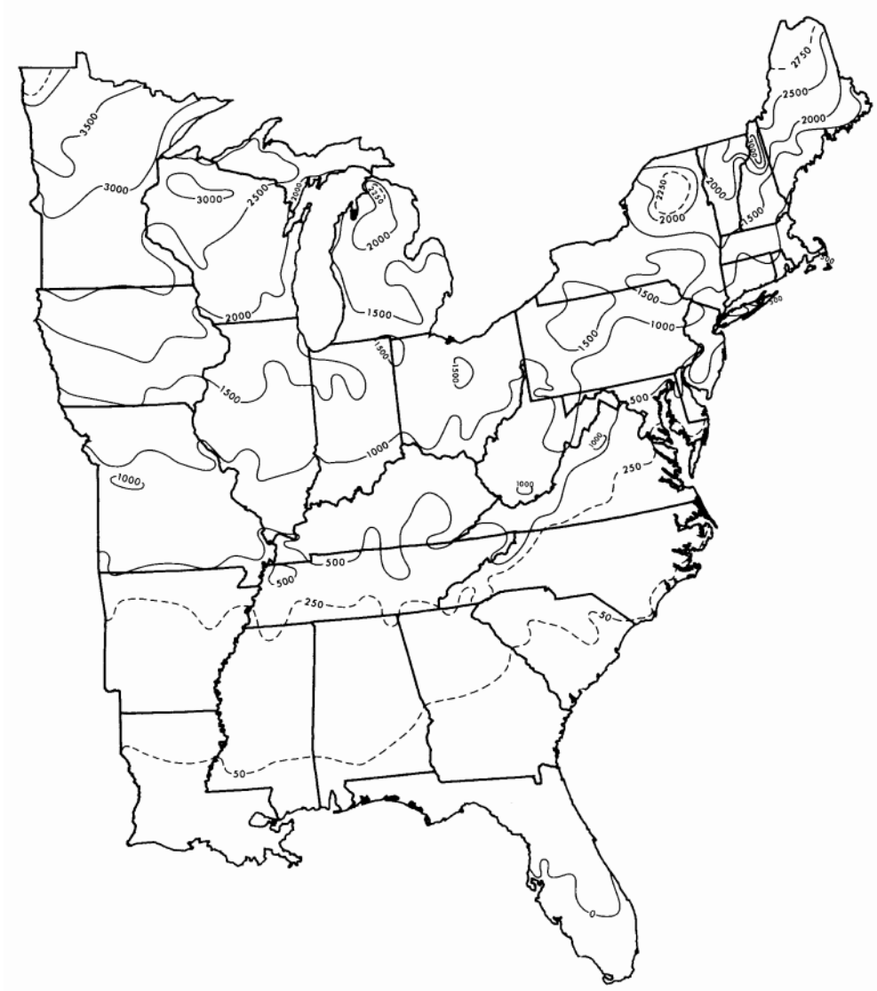
FIGURE A1, Continued. United States Design Air-Freezing Index (°F-Days) Contour Map (an Estimate of the 100-Year Mean Return Period), F_{100}
