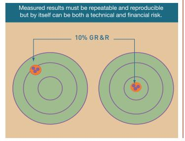
Measurement uncertainty is the quantitative evaluation of the reasonable values that are associated with a measurement result. It is a probabilistic expression of the doubt in a particular measurement value.
