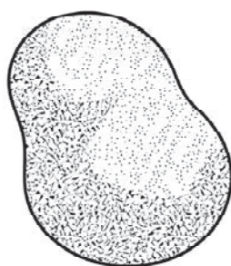
a) nanoparticle (3 ext. dimensions in the nanoscale)
