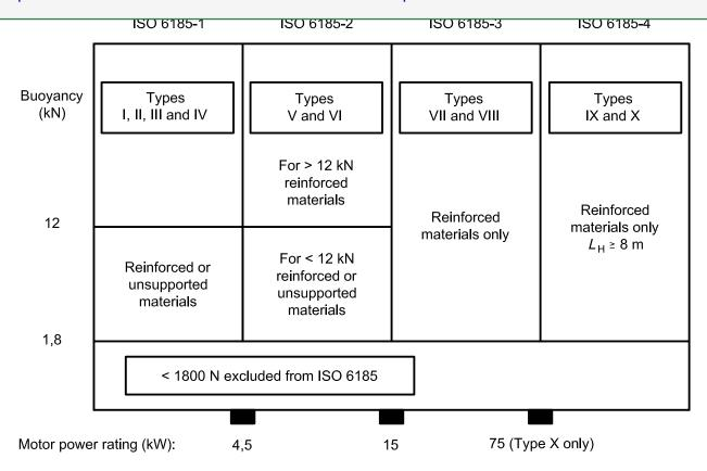
Figure 1 — Illustration of how ISO 6185 is subdivided
