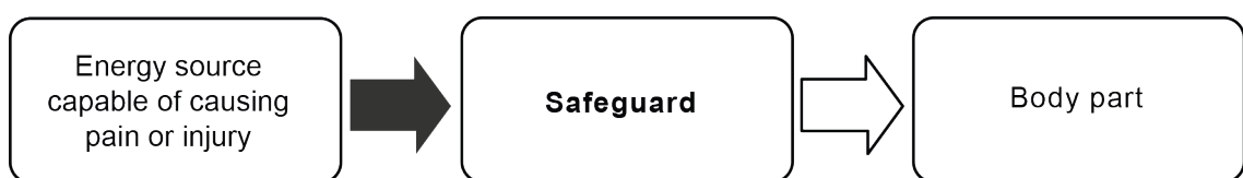
Figure 2 – Three block model for safety
