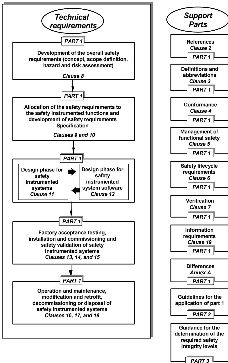
Figure 1 – Overall framework of this standard
