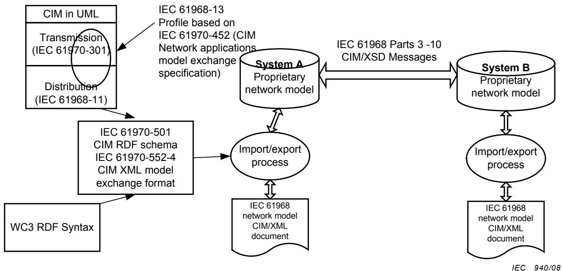
**Figure 1 – XML-based DMS network data configuration**
