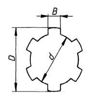
minor diameter d and the outside diameter D, these three numbers being separated by the sign  $\times$ ; for example :
