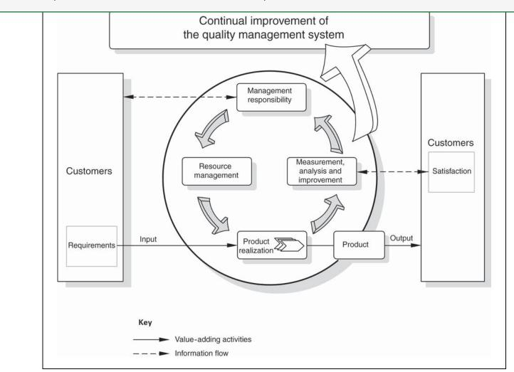
Figure 1 — Model of a process-based quality management system
