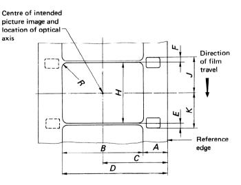
The film is shown as seen from inside the camera looking toward the lens with the photographic layer away from the observer.
