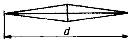
Figure 1 — Base area of the indentation produced by the Knoop indenter
