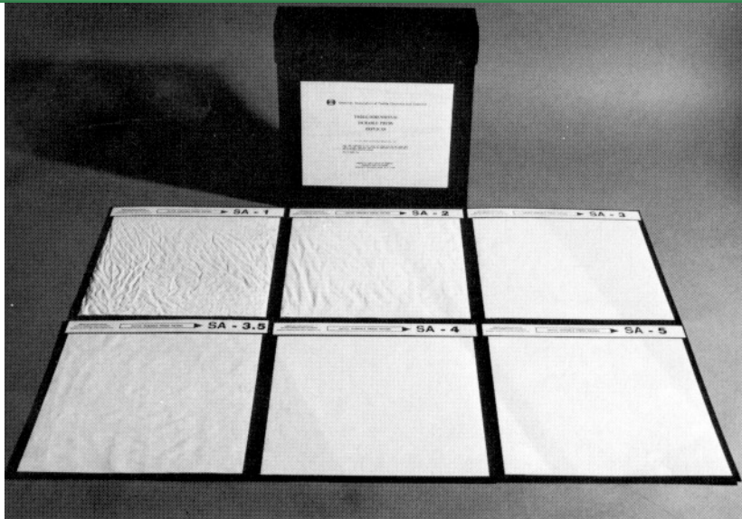
Figure 2 — AATCC wrinkle replicas for gradings (left to right, top to bottom) 1, 2, 3, 3,5, 4 and 5
