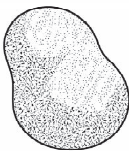
a) nanoparticle (3 ext. dimensions in the nanoscale)
