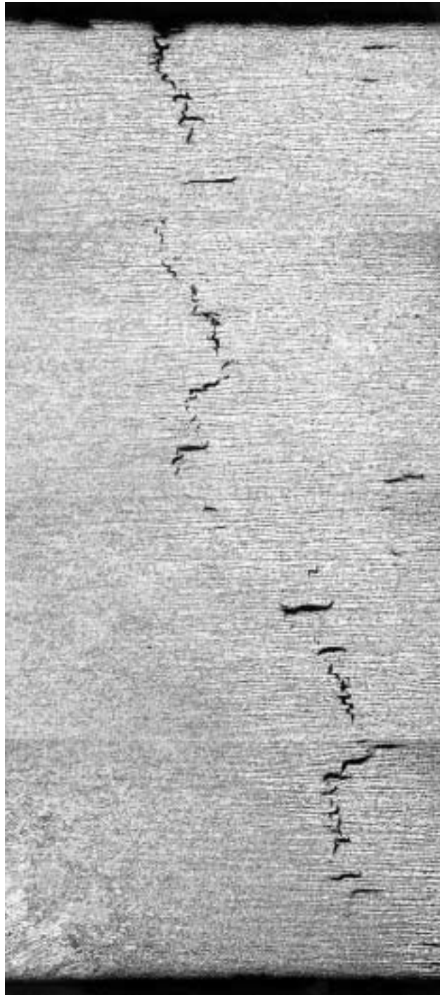
FIGURE 2—SOHIC in Carbon Steel Under Applied Stress. Direction of tensile stress is normal to cracks linking the blisters.
